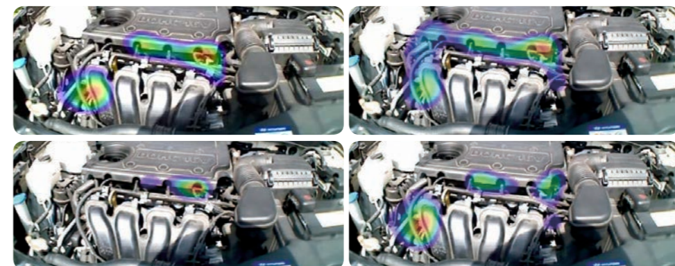
The detection of high frequency noises from a vehicle engine. [SeeSV-S205]
