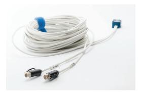
Each sensor cable is 23 feet long and terminates to a single triaxial connector. Pigtail or adapter cables are available to support a variety of termination options.
