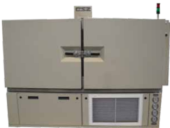
Front-opening freezer for epoxy storage
