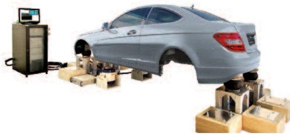
For maximum torsion, the body in white is connected at the extreme outer corners
