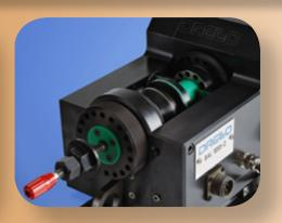
Optionally available insulated firing pinsenable triggering of a predefined measurement ( $t_o$  impulse). The exchangable breech head enables easy use of different firing pin shapes. The individually adjustable headspace and firing pin protrusion parameters enable checking of all types of ammunition in combination with the designated test barrels under various aspects.
