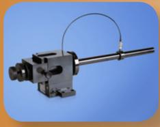
Devices of the 1055 series are used for testing ammunition. The barrel change system enables fast changing of barrels for different calibers. All test barrels can be supplied as velocity barrels, gas pressure barrels and precision measurement barrels.
