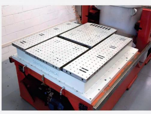
**Excellent Flexibility:** fast change of configurations, just removing fixing bolts and moving aside the table parts. Easy and clean operations to meet each specific requirement.
