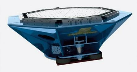
There is a perfect alignment between shaker armature motion and expander motion. The guidance is mounted and aligned on the machined frame, assuring precision and locking lateral and rotational expander modes. The guidance is completely mechanical, without oil or additional equipment, very low maintenance is therefore needed.
