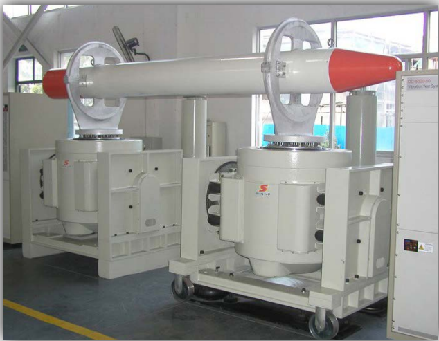
Dual Shaker Vertical Push-Push Arrangement
