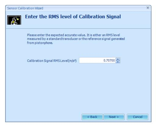
Now, the sensor is ready for calibration. Activate the excitation and press **Start Calibration**. After a few moments, the correct sensitivity will be calculated.
