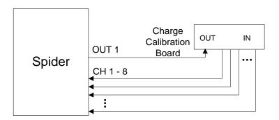
When everything is connected, select Tools -> Charge Calibration in EDM. The two charge ranges, 10,000 pC and 49,000 pC, must be calibrated separately. To choose the range to calibrate, select it under Calibrate Mode and then press **Set Charge Mode**. Then, run the calibration process by clicking **Start Charge**. The whole process is automatic and will complete within a couple seconds.
