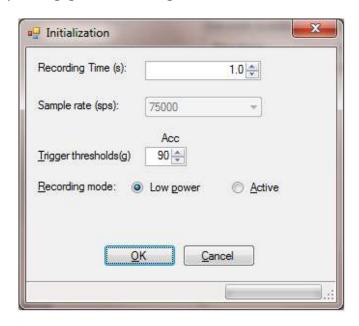
2. After clicking OK, a dialog box will tell you that the system is armed. You can then disconnect the TSR from the PC. The LED will flash blue at an increasing rate for about 30 seconds while it is in its arming and sensor warm-up phase. After the LED goes dark, the unit is armed. The TSR will trigger and collect data for the programmed period if the g threshold on any axis is met. The system will automatically re-arm for another event after the previous event recording is complete.
