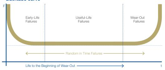
The ES altitude chambers allow the best cost effectiveness using the same chambers to perform vacuum and stress screening test that can force infancy failures that would otherwise occur after final assembly and product delivery, and potentially during the warranty period
