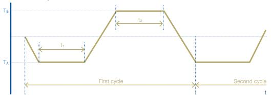
Stress screening ensures that defects, which normally arise during the product's useful life, are discovered during testing prior to the pre-production phase.
