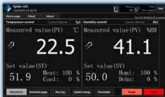
Test status page of EDC on a wireless, touchscreen terminal.
