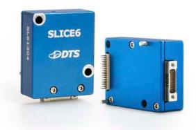
SLICE6 is an ultra-small, 6-channel data acquisition system. Originally designed to be integrated into crash and blast test ATDs, SLICE6 is ideal for applications with tight space constraints. SLICE6 offers direct-mount sensor solutions and supports a variety of sensor types including accelerometers, load cells, pressure sensors, IR-Tracc and potentiometers.
