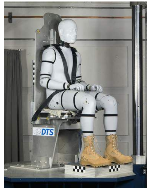
WIAMan with 146 SLICE6 HB channels
