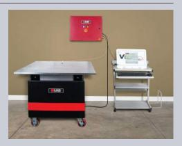
calculates the displacement with a known frequency and acceleration and then manually adjusts counter-weights on the vibration table to deliver the calculated displacement.
