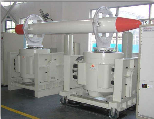
Dual Shaker Vertical Push-Push Arrangement
