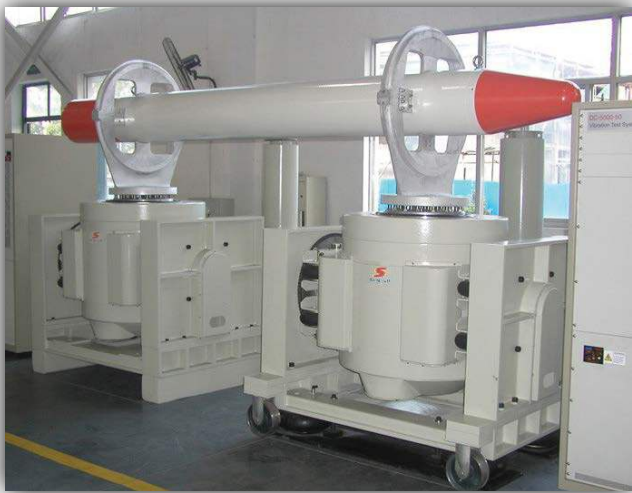
Dual Shaker Vertical Push-Push Arrangement
