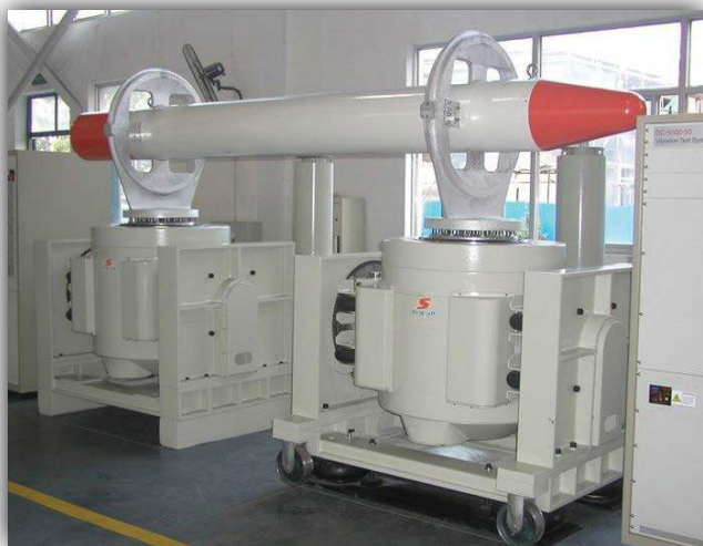
Dual Shaker Vertical Push-Push Arrangement
