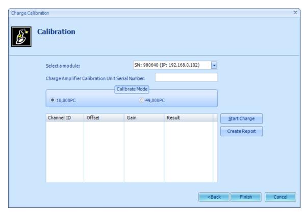
The results will be shown in the table. For each channel, if the gain error is within the acceptable range the result will show as "Pass". Press **Finish** to complete the calibration and accept the changes.
