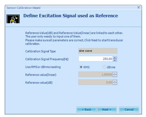
The signal reading, which is the RMS or dB amplitude of the sensor excitation, is entered here.
