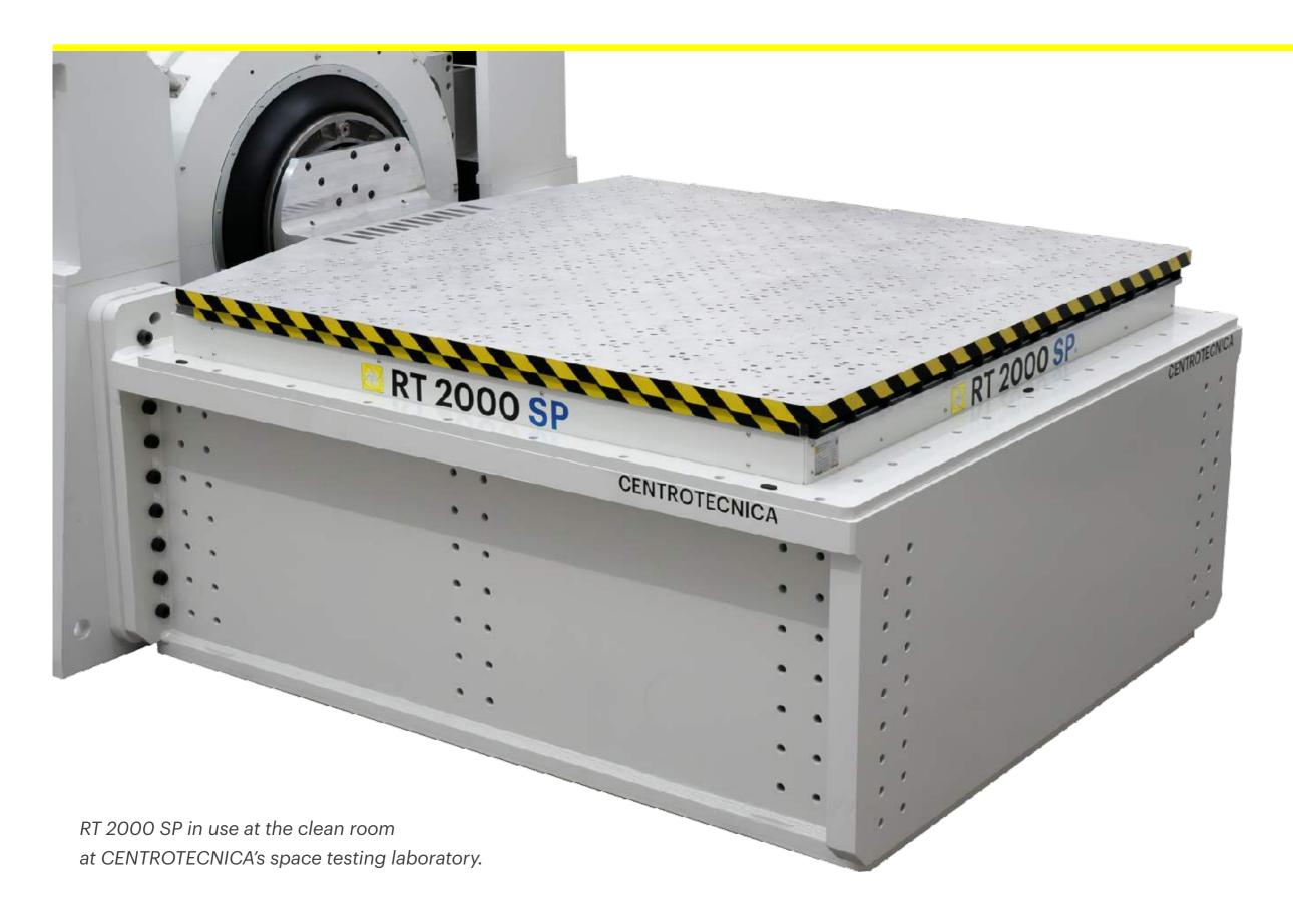
RT series slip tables are equipped with a fully mechanical, **OIL-FREE** guiding system, a feature that eliminates the risk of DUT contamination. This feature is particularly appreciated by space-sector customers testing in clean room.
