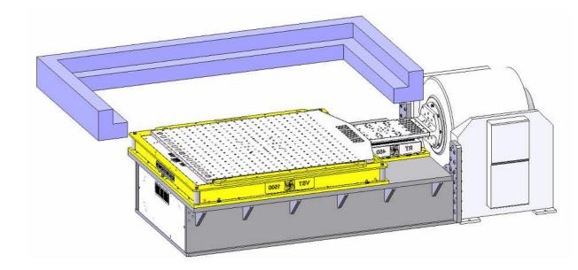
The slip table with double driver bar allows for in-line working of 2 opposing shakers.
