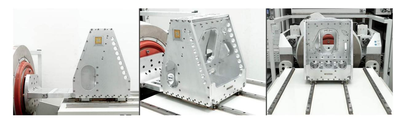
CENTROTECNICA has taken the concept of weight saving to the extreme by developing the RT fixture solution: fixtures that mount directly onto the RT slip table rails, eliminating the need for a table.
