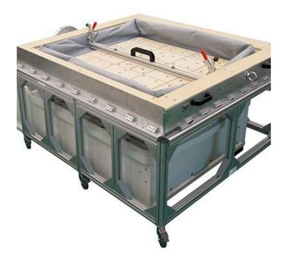
**Direct Coupling Solutions:** quick coupling system between climate chamber and slip table to take full advantage of the flexibility of slip tables (not just RTs).
