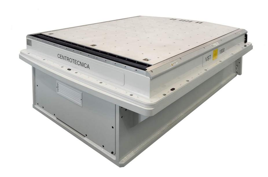
**VST**: hydrostatically supported product, it uses vacuum force as the drive system. It offers very high performance due to exclusive, patent-protected technology. The benefits offered by this product are most noticeable with large slip tables.
