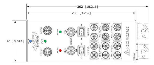
The LED indicators make it easy to see when the system has sufficient power, whether high voltage is present, and the status of the built-in SLICE6 data acquisition system.
