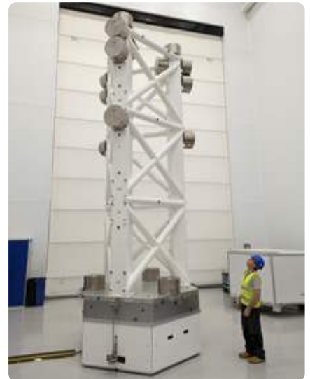
System with precisely known mass properties used for accuracy checks (Resonic 6000F)
