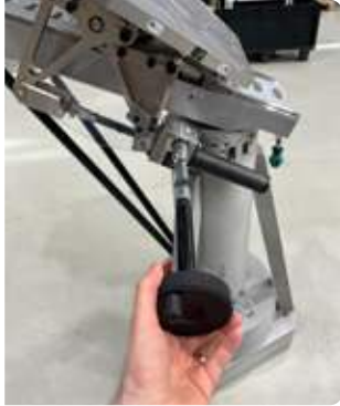
Up to 80 kg: Resonic P. The platform is moved by spindles.
