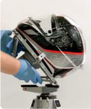
Up to 20 kg: Resonic K. The platform is moved by hand.
