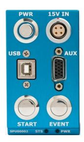
**15V IN** power input connector - 9-15 VDC; 1.7 A minimum
