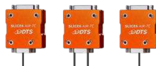
SLICE6 AIR-TC data acquisition unit with three TC Interface blocks, shown as a 24-channel system
